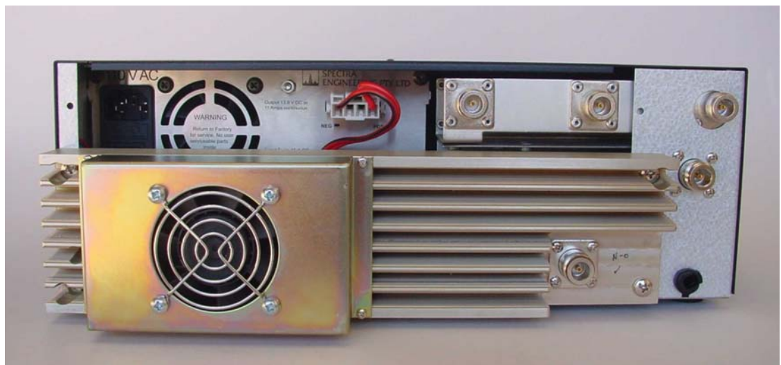
Figure 1-2 MX920 Rear Panel with Power Supply and Duplexer fitted. (RF Connecting cables not shown)
