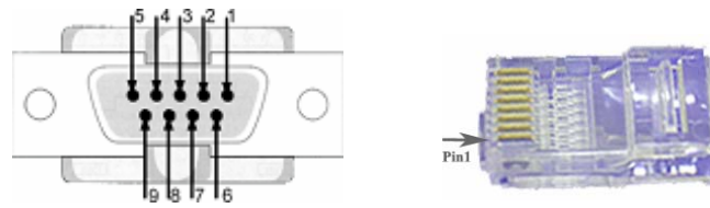
Figure 8-2 Front view of DB9 female connector and RJ45 Modular male connector
